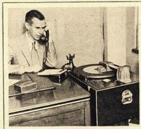
No more office secretaries? This device answers the telephone for you when you are out and announces the hour of your return.
